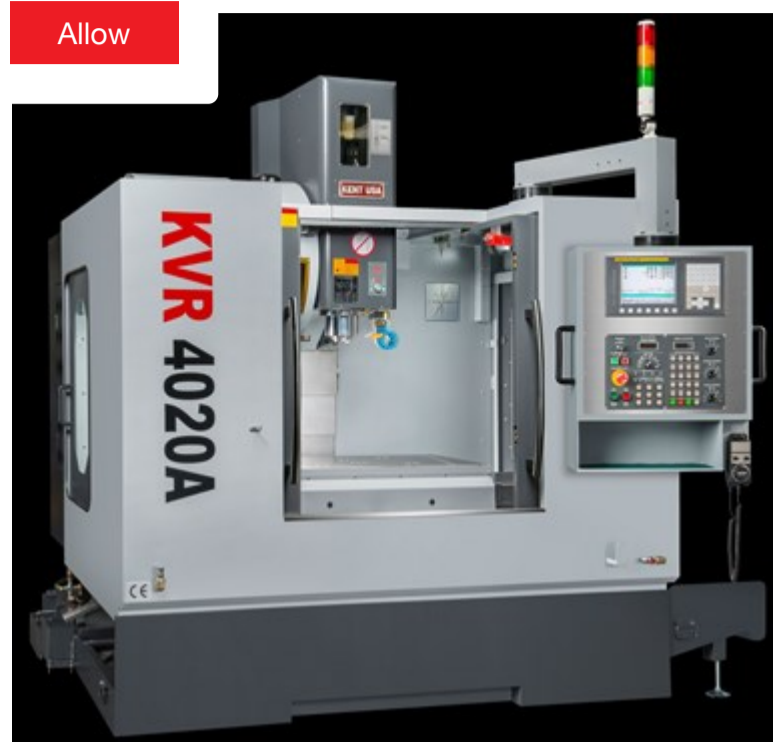
The medium-duty KVR 4020A linear way VMC series is pre-wired for a fourth axis, which has increased Mega Industries’ flexibility.
