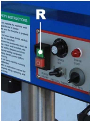
Figure 7-1: Main Power ON
