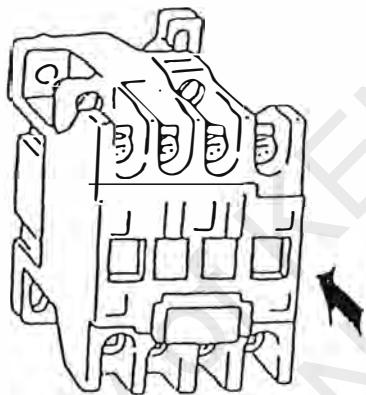
When the magnet switch is activated, the movable spring support is extracted approximately 4mm from the switch body.
