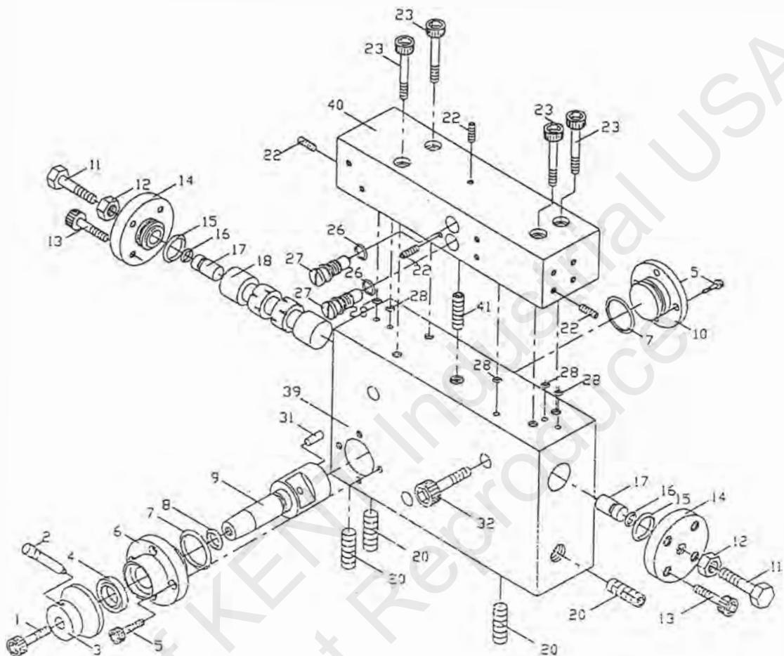
3.10.2 List of parts for mechanical/proximity type of hydraulic valves
