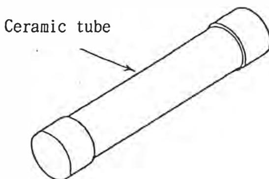
Cartridge fuse contains its fuse element in a transparent glass-tube or ceramic tube.
